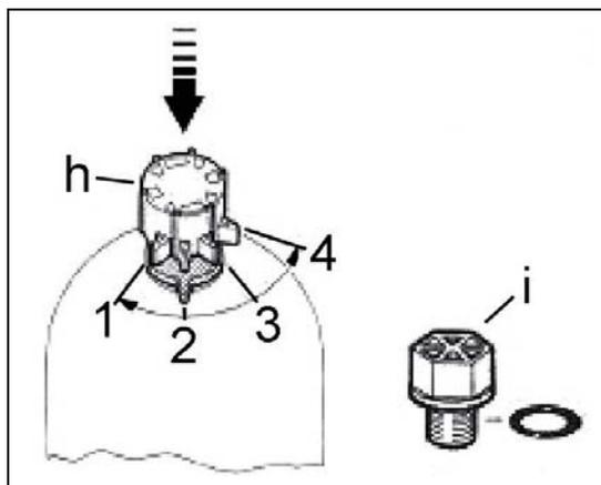
To regulate the output quantity or the droplet size, the spray pressure can be adjusted in steps from 1–4 bar [14.5–58 psi].
