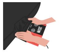
Stretch Tube Around Heating Unit (Observe "Do Not Cover" markings)
